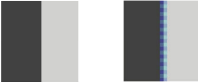
Fig. 2: Zipper artifacts on a vertical line (CHANG 2006)
