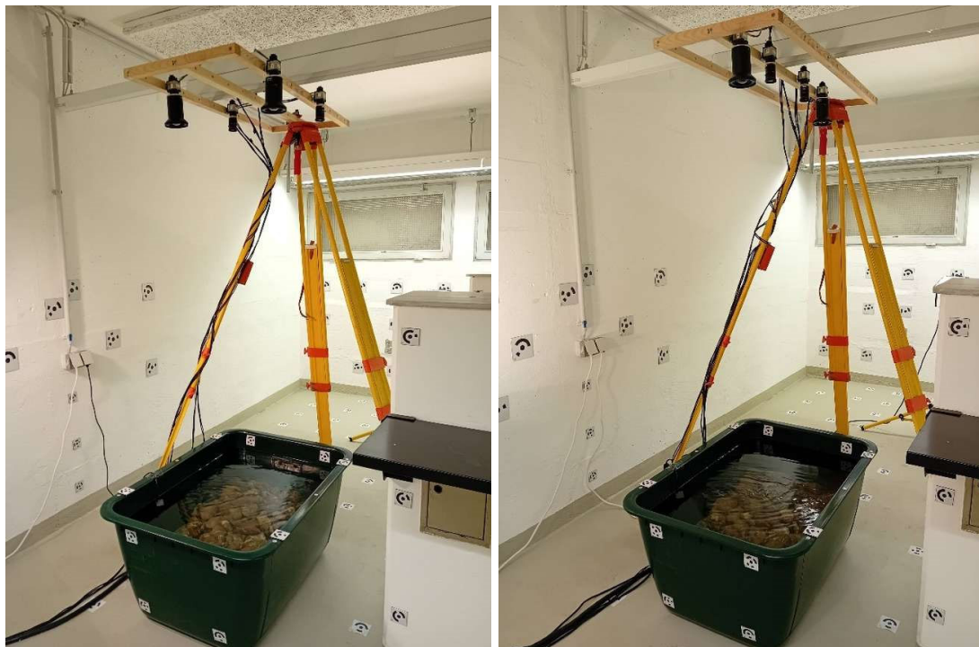
Fig. 5: Implementation of the experiment in the lab (left) and photo of the water tank, the topography and a dynamic water surface generated by a pump (right)
