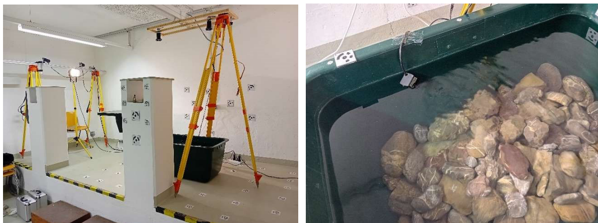
Fig. 2: Implementation of the experiment in the lab (left) and photo of the water tank, the topography and a dynamic water surface generated by a pump (right)
