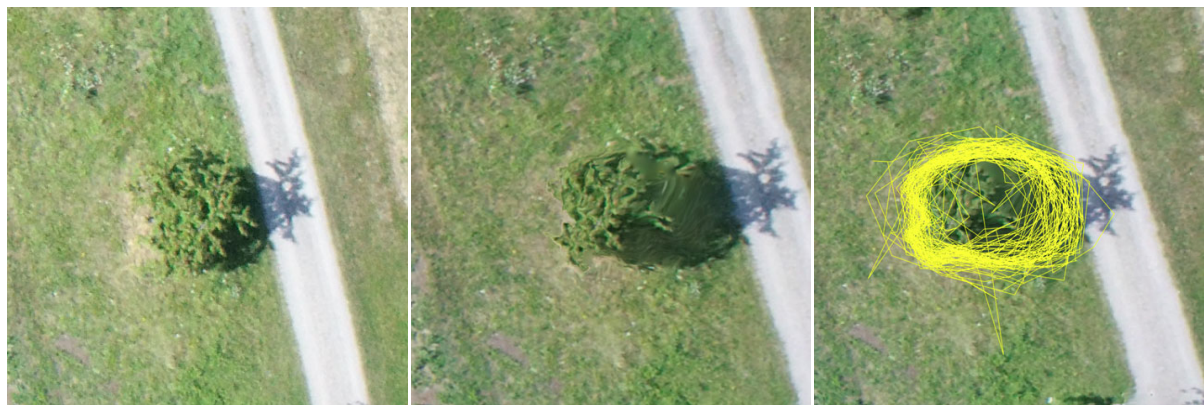
Fig. 3: From left to right: raw drone image, ortho-image and the geometries collected by crowdworkers on the ortho-image. Mainly caused by the shadow, at the right side of the tree, blurring occurs due to the ortho processing. Thus, it is harder to distinguish between the ground and the tree resulting in a higher variation of the annotations in this part of the tree.
