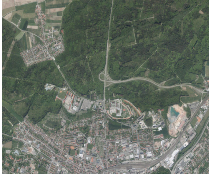
Fig. 1: Simulated satellite image with mismatching line rate at 4 m GSD derived from DOP40
