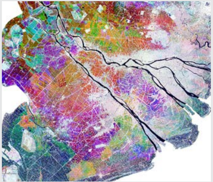
This multi-temporal false color composite of the Mekong River, located in Southeast Asia, shows different stages of crop growth. The source image is Sentinel-1, processed using ENVI SARscape by sarmap SA.
