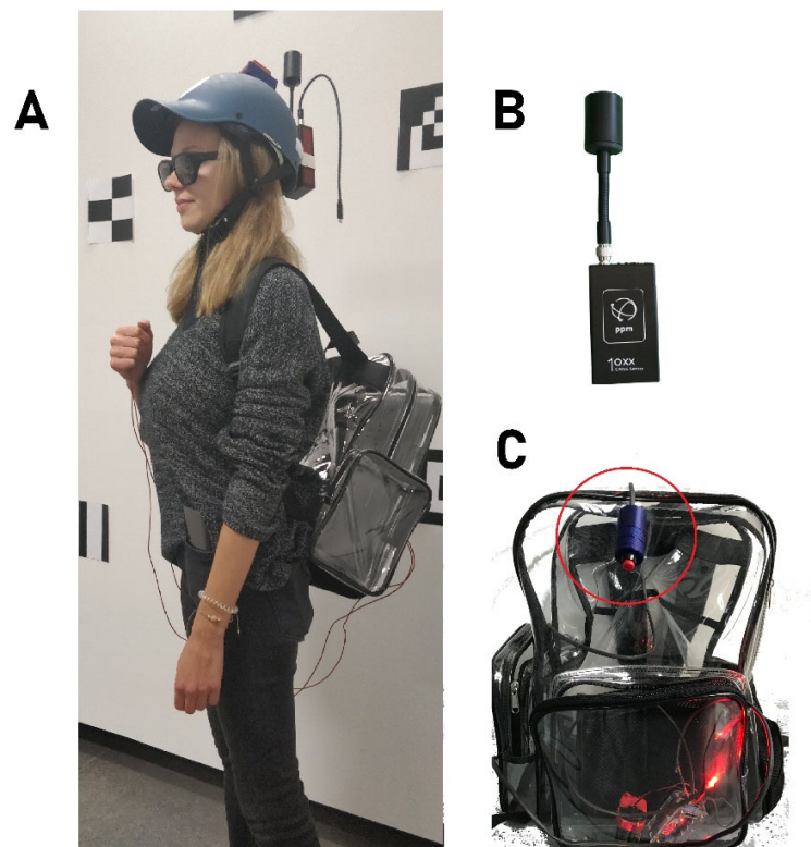
Fig. 1: A: A sample participant in full equipment. B: GNSS receiver (PPM 10-xx38). C: During the experiment, participants requested navigation instructions using a custom-built clicker-device (circled in red) which triggers a LED light located in the backpack informing the experimenter about the request.
