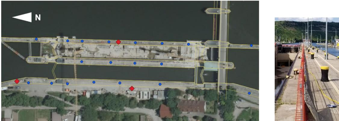
Fig. 3: Test area of ship lock Hessigheim/Neckar with distribution of signalized points. The image on the right shows one of the signalized points. All points are fixed to the ground except three, which are mounted on top of approximately 140 cm high concrete pillars (red squares).
