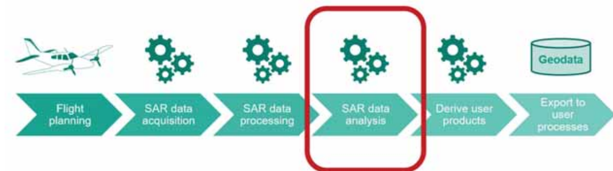
Fig. 1: Development chain, including flight planning, data acquisition, processing and analysing as well as generating and providing geodata products.
