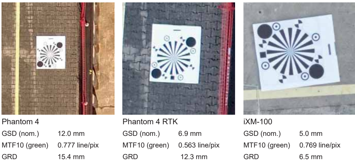
Fig. 1: Siemens star image and analysis from Phantom 4 (left), Phantom 4 RTK (middle) and Phase One iXM100-RS (right). Each image sample is sized 300 x 300 pix.
