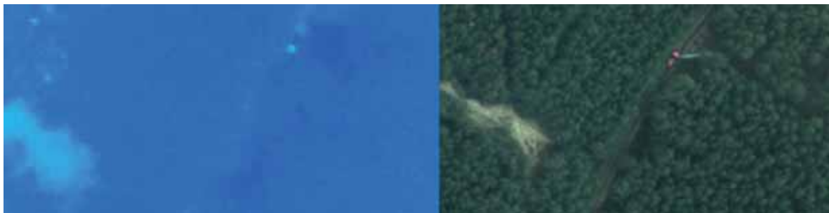
Fig. 7: Zoom into Fig. 6: Colder areas (dark blue) can be nicely explained using in the high resolution RGB image, they are caused by watering the adjacent forest by fire trucks
