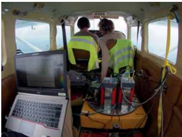
Fig. 1: Operation of 4-head camera system on stabilizing platform
