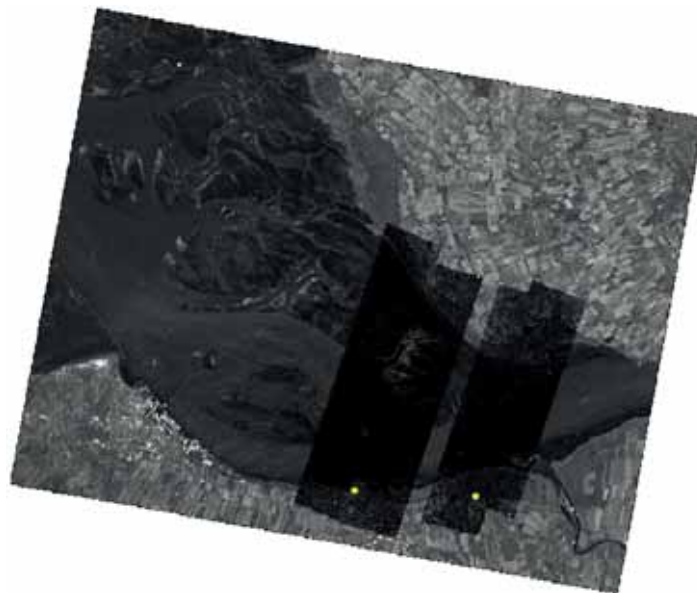
Fig. 3 TerraSAR-X image overlaid by F-SAR data strips and marked reflector positions
