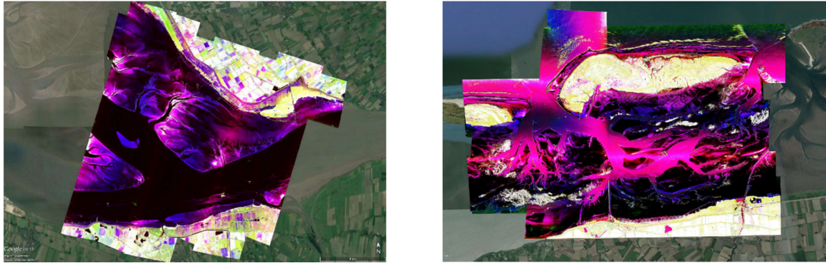
Fig. 1: Polarimetric S-band SAR image mosaic, captured over the Medem channel (left) and Otzumer Balje (right). In the background, an image of the corresponding region from GoogleEarth is displayed
