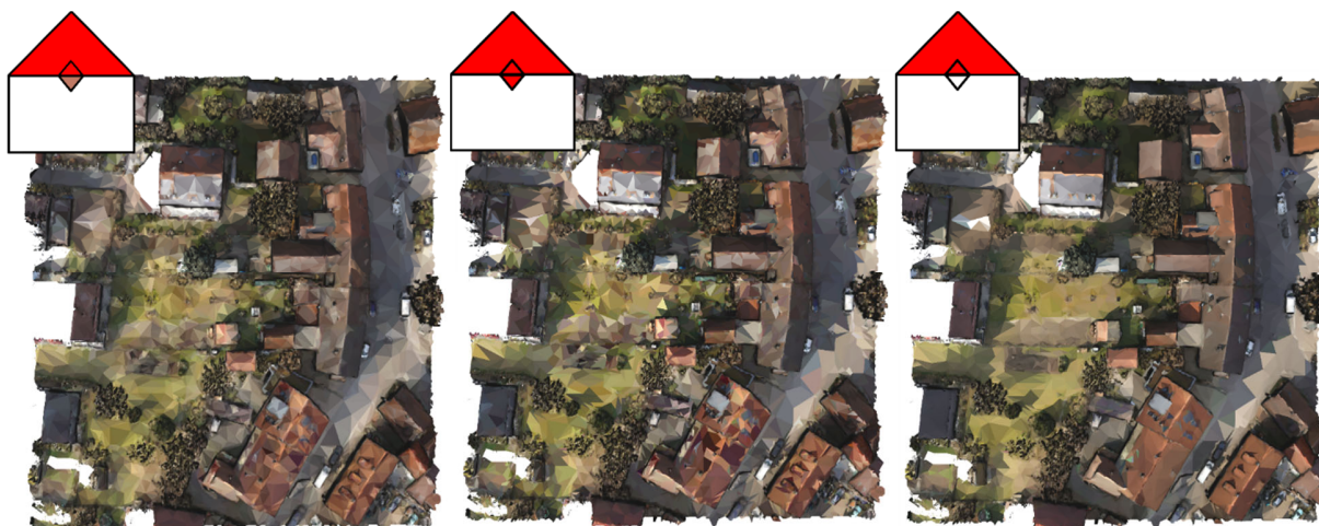
Fig. 3: Comparison of radiometric features at different qualities in RGB color space. The faces are colored based on mean/median RGB values. Quality of radiometric features increases from left to right. Left : Mean RGB of vertices, center : median RGB of vertices, right : median RGB of all pixels per face. A schematic drawing is attached to each subfigure in the upper left.
