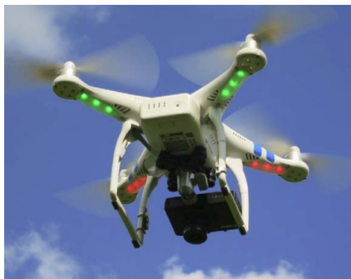
Fig. 2: DJI Phantom 2 equipped with Canon Powershot 110 (BARETH et al. 2015)
