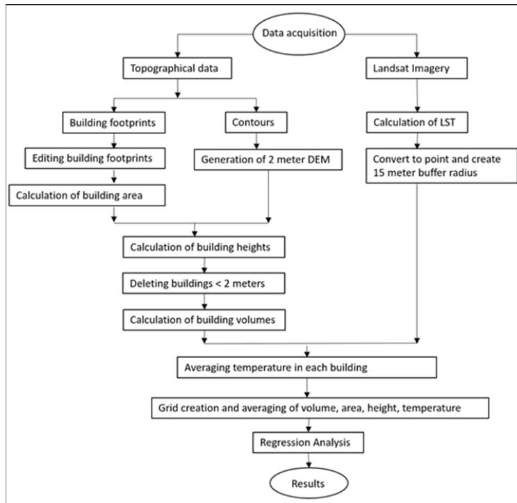
Fig. 2: Methodology framework for topographical datasets and LST
