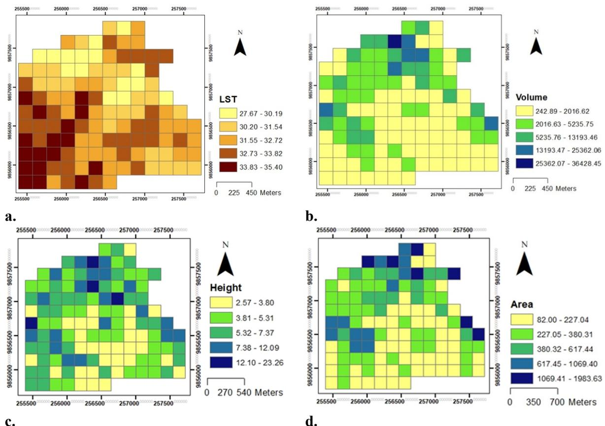
Fig. 6: Spatial distribution of LST (a), building volume (b), area (c) and height (d) in the grid
