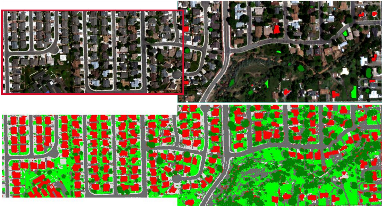
Fig. 4: Softmax Regression classifier: Merge of two classification images (bottom). The classifier was trained on one attribute image (top right) and then applied to a similar attribute image (top left)
