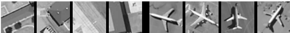
Fig. 5: Training of the Deep Learning network for recognition of commercial airplanes with negative (left) and positive (right) training chips
