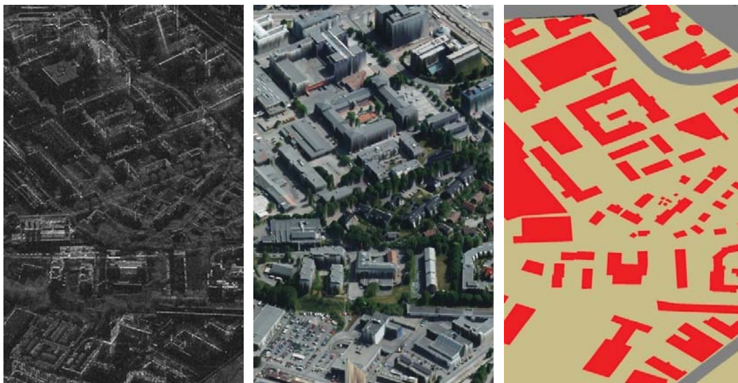
Fig. 5: Example of co-registration results obtained with the described approach: SAR image of a small area of the city of Oslo (left), co-registered optical image (center), and GIS data showing the location of building footprints in red and roads in dark gray (right)
