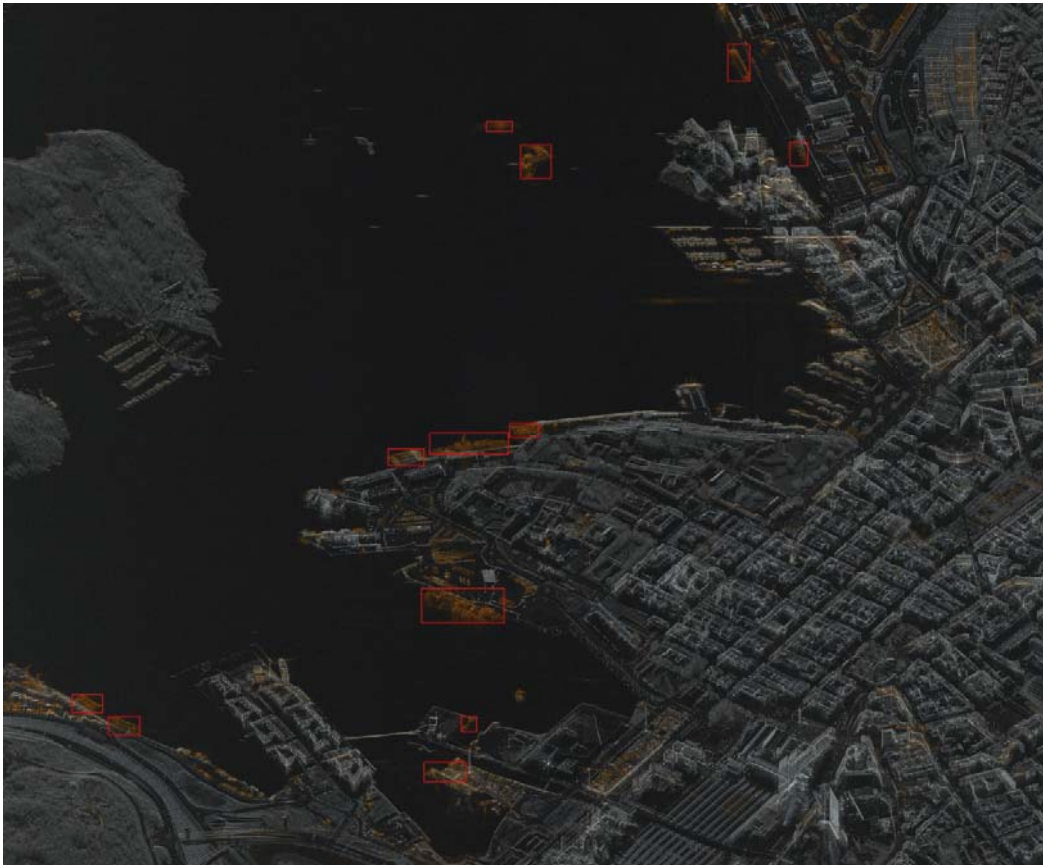
Fig. 7: Results of applying the proposed workflow for detecting ships that arrived/left the port of Oslo. Red rectangles show the ships that were automatically detected. For easier visualization, the rectangles are drawn over a RGB composite of two TerraSAR-X images that highlights the changes in orange
