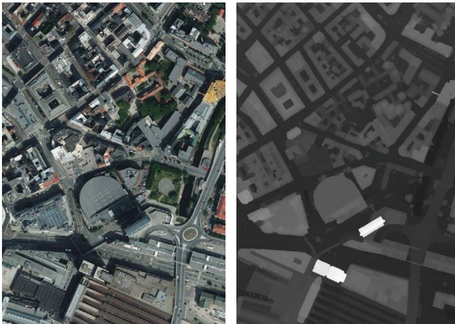
Fig. 2: True orthoimage (left) and DSM (right) from a small area near the Oslo train station, obtained from a set of optical images by using the approach described above
