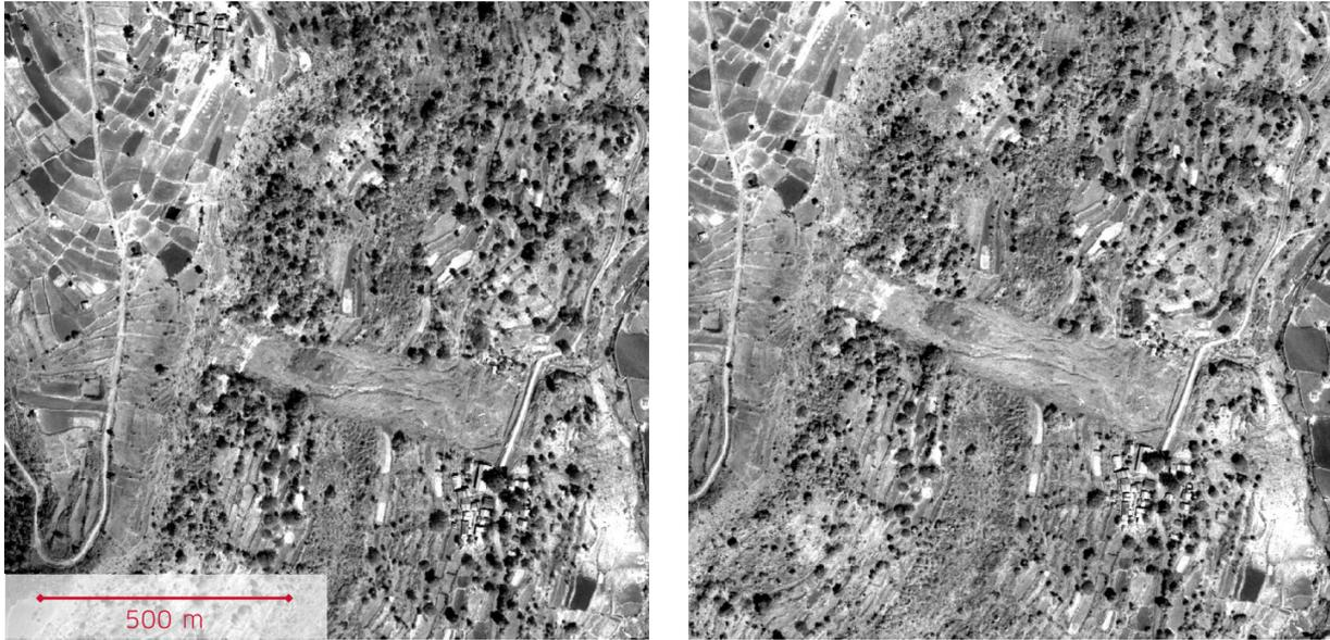
Fig. 1: Pléiades panchromatic stereo pair of the Malin landslide area, used to run the photogrammetric generation of a point cloud from optical imagery (subset, GSD 0.5 m).
