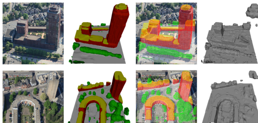
Fig. 3: Reconstruction with and without class-specific priors. Left to right: example image; semantic reconstruction; semantic reconstruction back-projected to the image; and generic volumetric surface reconstruction with the same input (Zach 2008).
