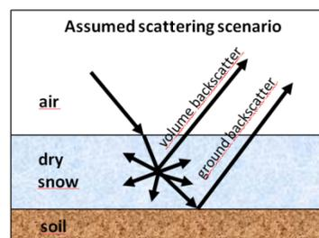
Figure 3 Simplified scattering contributions from a dry snow pack on ground (after ROTT et al., 2010).
