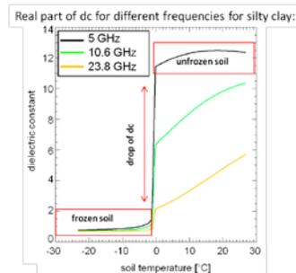
Figure 5 Modelled behaviour of the real part of the soil dielectric constant in dependence of soil temperature after ZHANG et al. (2003) for three different frequencies. For the C-band region the black 5GHz curve is applicable.
