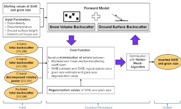
Figure 2 Inversion procedure for retrieving the snow water equivalent.
