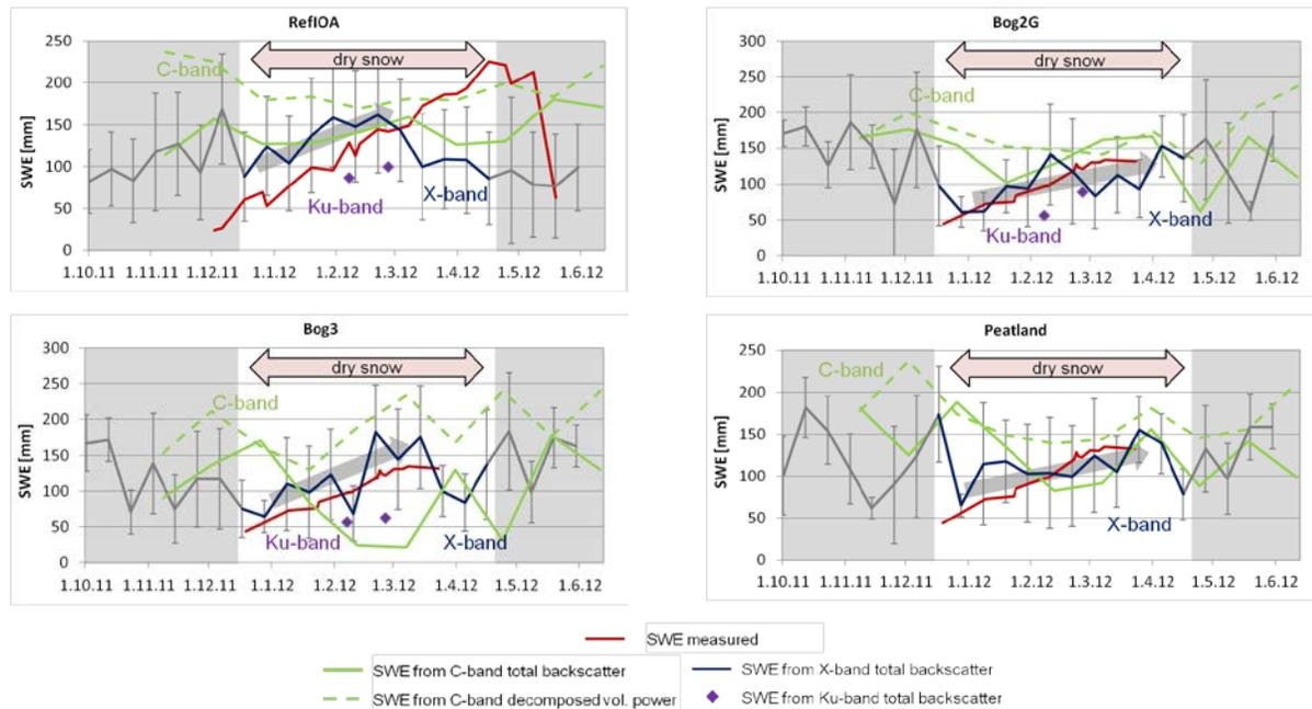
Figure 4 SWE inversion results for C-, X- and Ku-band from all four inversion scenarios compared to measured SWE values (red). Grey bars to both sides indicate the invalid areas for SWE inversion due to mainly wet snow conditions or lack of snow at the end of the winter period.
