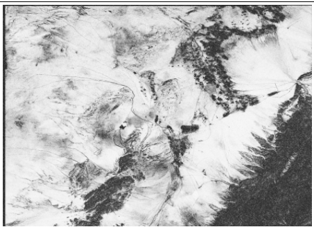
Interseismic pair of the Bam (Iran) region: Long-term interferometric coherence (baseline: 498.2m, time difference = 175 days)
