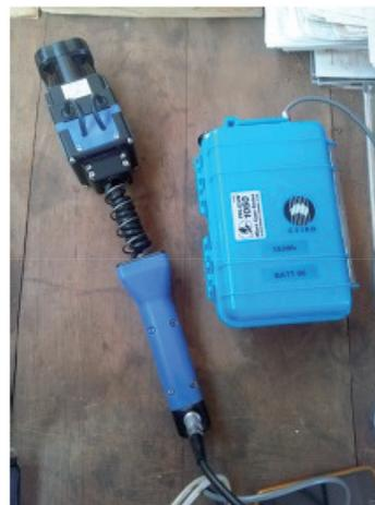
**Fig. 1:** Zebedee scanner and its associated hardware.
