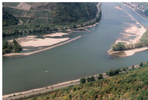
Fig. 13: Dry fallen areas with groynes und groyne fields of river Rhine near Kaub.
