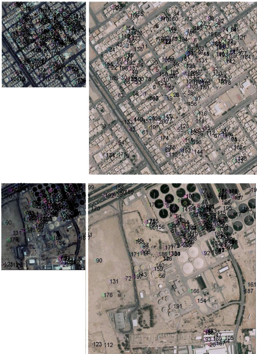
Fig. 5: Distribution of matched points for left (built-up) and right (built-up/open) image patch of the upper row shown in Fig. 4 (left IKONOS image, right: orthophoto).
