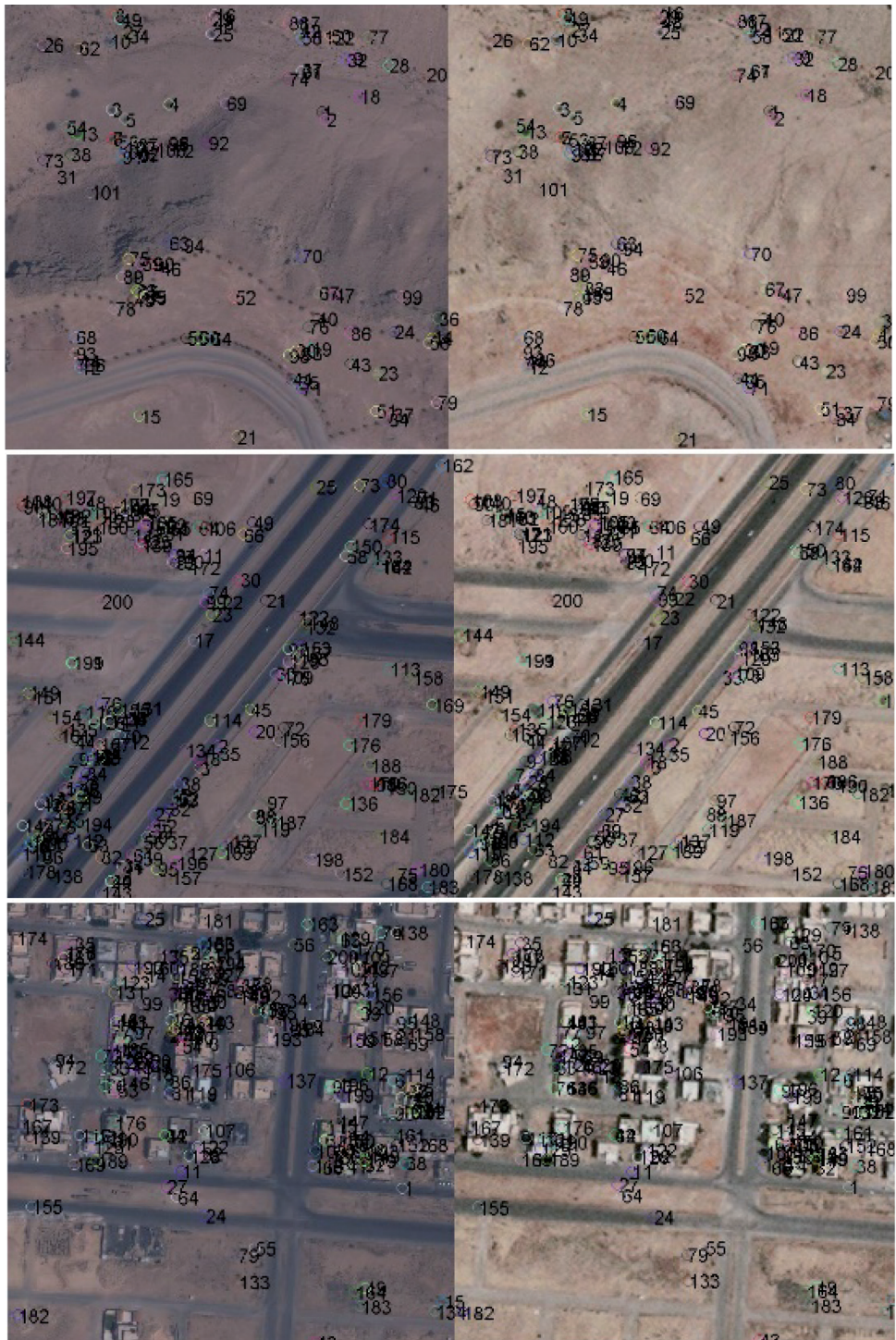
Fig. 3: Distribution of matched points for three selected image patches (left GeoEye image, right orthophoto) shown in Fig. 2: left patch of upper row (open), centre patch of middle row (built-up), centre patch of lower row (built-up).
