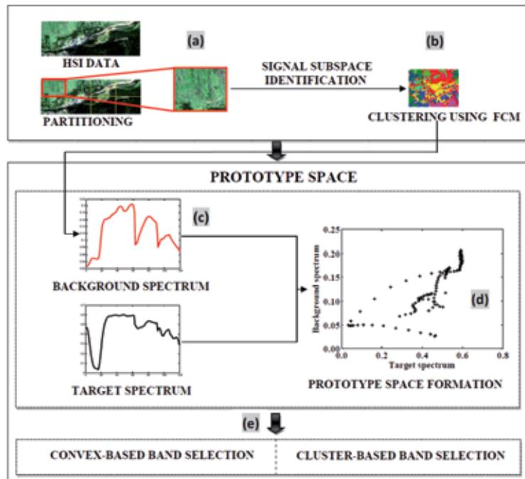
**Fig. 1:** Block diagram of the proposed local band selection approaches in the PS: (a) image partitioning, (b) data clustering, (c) determining the background spectra, (d) prototype space formation, and (e) band selection.
