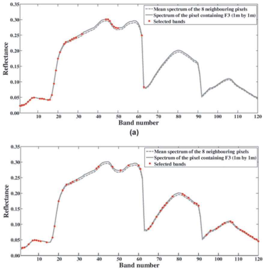
Fig. 4: Representing selected bands in the spectral space: (a) convex-based band selection, and (b) cluster-based band selection. Red dots show the selected bands.
