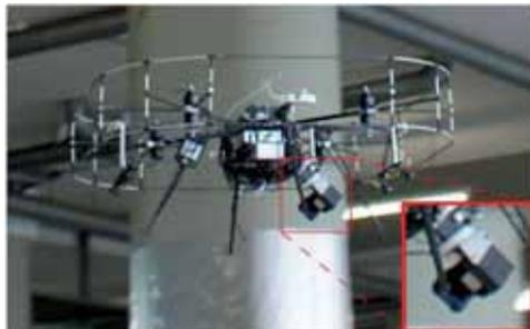
**Fig. 1:** The 3D laser scanner mounted on our MAV.
