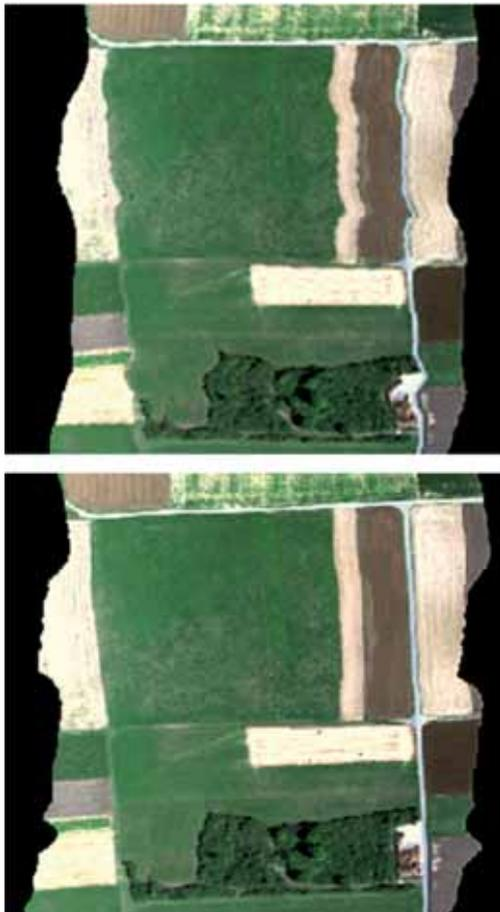
**Fig. 12:** Direct georeferencing based on GPS/IMU (top) and exterior camera orientation (bottom).
