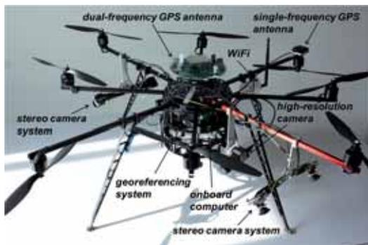
**Fig. 1:** The MAV (modified OktoXL, HiSystems) including the sensor and processing components, developed within the project *Mapping on Demand*.
