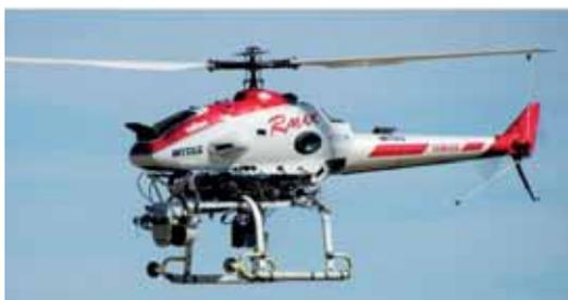
Fig. 1: The UAS Tech Lab RMAX helicopter.
