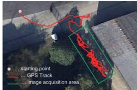
**Fig. 7:** The RTK-GPS positions during the test flight. Images were taken in the image acquisition area to observe the building on the right.
