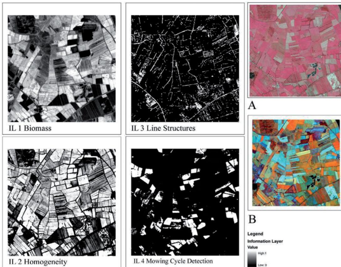
**Fig. 4:** Information layer (IL1-4) examples based on aerial orthophotos (A = DMC camera with 0.4 m ground sampling distance GSD and four channels) and satellite data (B = RapidEye, 5 m GSD, 5 channels).
