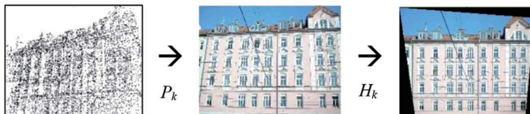
Fig. 1: Projection and homography matrix for mapping 3D points and pixels of the rectified image.
