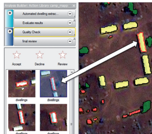
Fig. 2: Hybrid solution for a combined automated and manual analysis and quality check, programmed in eCognition Architect. Extracted dwellings are visualized as thumbnails for an easier post-processing and editable as well as linked to the object in the image scene.
