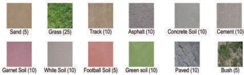
Fig. 3: Examples for targets ( 1 \times 1 \text{ m}^2 ) in the check areas and the number of reflectance values derived from spectrometer measurements per check area between brackets. As there are five measurements per target, the number of targets per check area is the number of measurements divided by five. For instance, there was one target over sand, but five targets over grass.
