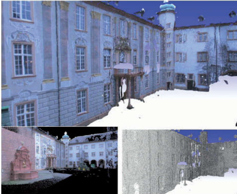
Fig. 8: Top: Textured preliminary result for 3D surface reconstruction of the facade of Ettlingen castle. Bottom left: Dense 3D point cloud. Bottom right: Shaded 3D surface with wire frames. The results base on the image-sets ‘fountain-R25’ and ‘castle-R20’ of (STRECHA et al. 2008).
