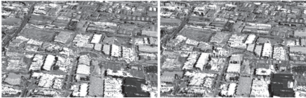
Fig. 8: Perspective 3D visualization of original DSM (DSM_C1, left) and enhanced DSM (ENH_HYB, right), both with vertical exaggeration 2.0, texture with C1 orthoimage (2.5 m).
