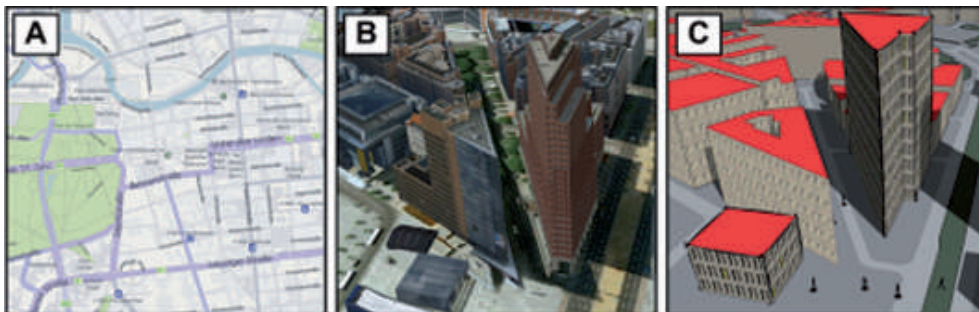
Fig. 2: Comparison between (A) digital 2D maps and virtual 3D city models rendered with (B) photorealistic rendering techniques, and (C) non-photorealistic rendering techniques.
