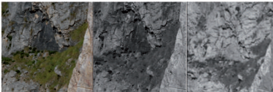
Fig. 1: Detail of a Nikon D200 photo; left: RGB; middle: greyscale; right: the corresponding part of a HySpex image, 1.629 \mu\text{m} wavelength.
