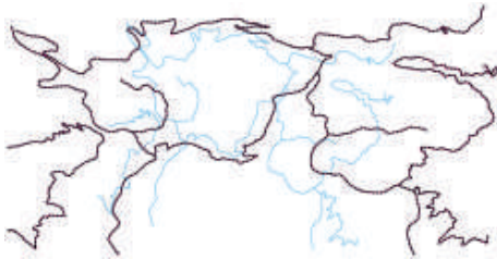
Fig. 7: Matching results of Test B1. The 3D GCLFs are extracted from a recent orthoimage.
