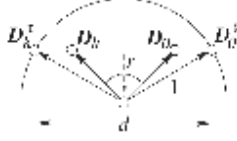
Fig. 3: Enforcing the Plücker constraint onto a 6-vector \mathbf{L}^\tau = [\mathbf{L}_h^\tau; \mathbf{L}_0^\tau] . Starting from vectors \mathbf{D}_h^\tau = \mathbf{N}(\mathbf{L}_h^\tau) and \mathbf{D}_0^\tau = \mathbf{N}(\mathbf{L}_0^\tau) , which in general are not perpendicular, we easily can enforce the perpendicularity by symmetric linear interpolation, leading to \mathbf{D}_h and \mathbf{D}_0 , which are perpendicular. The vector \mathbf{M} = \mathbf{N}([\mathbf{L}_h | \mathbf{D}_h; \mathbf{L}_0 | \mathbf{D}_0]) yields a valid Plücker vector close to \mathbf{L}^\tau .
