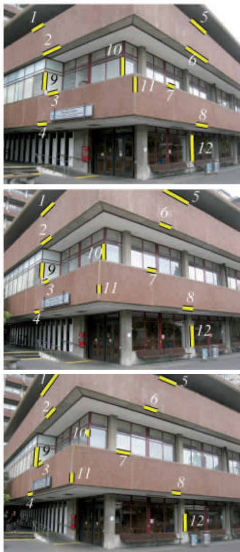
Fig. 4: Three images with 12 corresponding straight line segments used for the reconstruction of the 3D lines, forming three groups [1...4], [5...8], [9...12] for three main directions.
