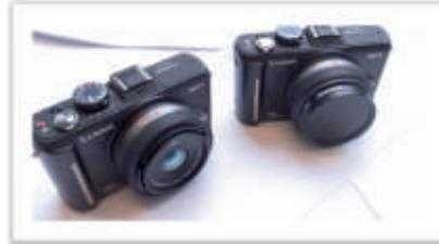
**Fig. 1:** Left: VTT hyperspectral camera UASI (SAARI et al. 2011). Right: Panasonic Lumix GF1 cameras.
