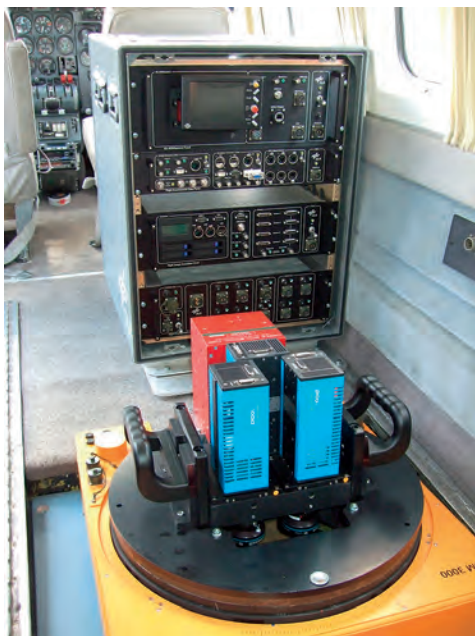
Fig. 5: MACS 50/70 on board an aircraft with data acquisition unit, GNSS/INS system, stabilized platform and peripheral equipment (without wiring).
