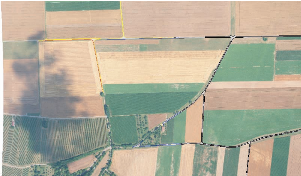
Fig. 11: Orthoimage mosaic B: Result of road-tracking started from the right (black), derived road parts up to required new initializations are color-coded (blue, red, yellow).
