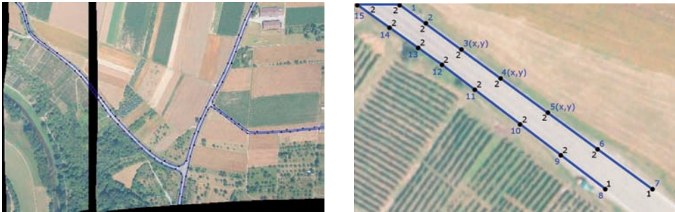
Fig. 2: Road outline superimposed on two images (left); detail properties of graph (right): node id (blue number), node degree (black number).
