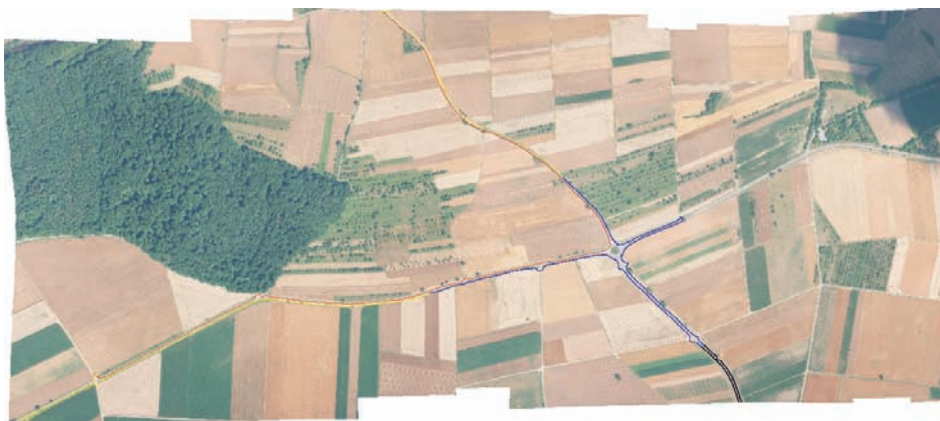
Fig. 8: Orthoimage mosaic A: Result of road-tracking started from the right (black), derived road parts up to required new initializations are color-coded (blue, red, yellow).
