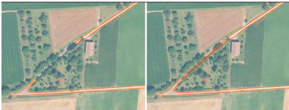
Fig. 14: Post-processing by topological connection of occluded road-sections: Stop at complete occlusion (left), connection through post-processing (right).
