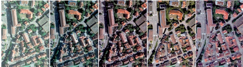
Fig. 3: Aerial images of Area 1 “Inner City” at individual flying times: from left to right: ‘08-07-24 RMK, ‘08-07-24 DMC, ‘08-08-06 DMC, ‘08-08-06 DigiCAM and ‘08-09-11 UltraCamX.
