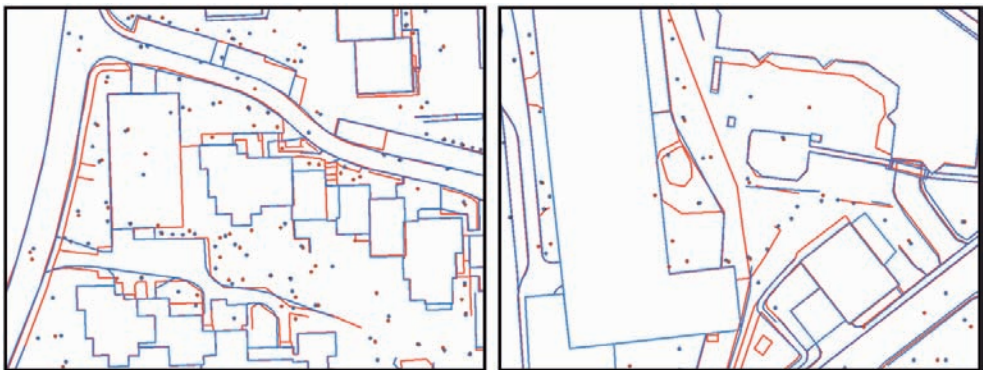
Fig. 7: Left: Area 2 "High Riser", comparison of stereoplotting results 8 cm GSD (red) to 20 cm GSD (blue), RMK. Right: Area 1 „Inner City“, comparison of stereoplotting results 8 cm GSD, UCX (red) to DMC (blue).
