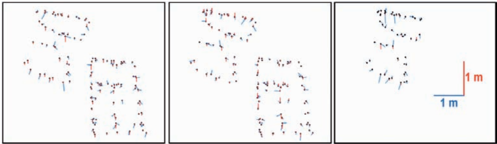
Fig. 9: Differences of all point measurements for Area 2 and 3 in 8 cm GSD. From left to right: RMK-DMC, RMK-UCX and RMK-DigiCAM (only northern Area 2). Differences dx and dy (blue), dz (red).
