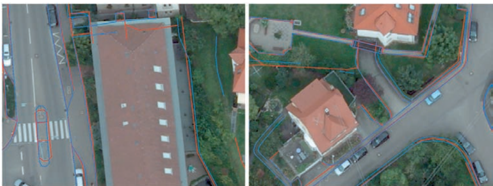
Fig. 11: Line measurements in 8 cm GSD images for RMK (red) and DMC (blue). Background image: UCX orthophoto, 8 cm GSD.
