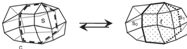
Fig. 3: A 3D Euler operation: splitting a solid s into solids s_0 and s_1 by the insertion of a 2D face f , and the inverse merge operation. The location of the contact between the face f and the boundary of the solid s is defined by the loop c .
