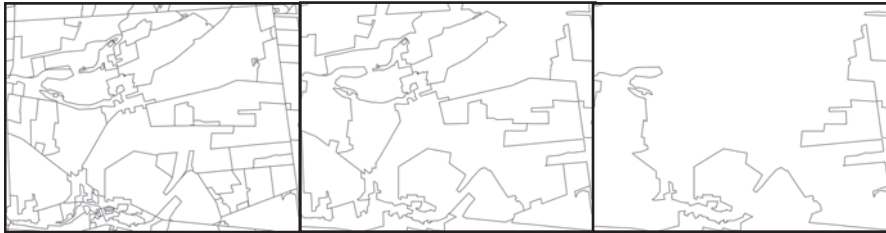
Fig. 9: Application example: a section of ca. 2% of a digital map on land-use at three different scales (by courtesy of J. HAUNERT, IKG Hannover University).
