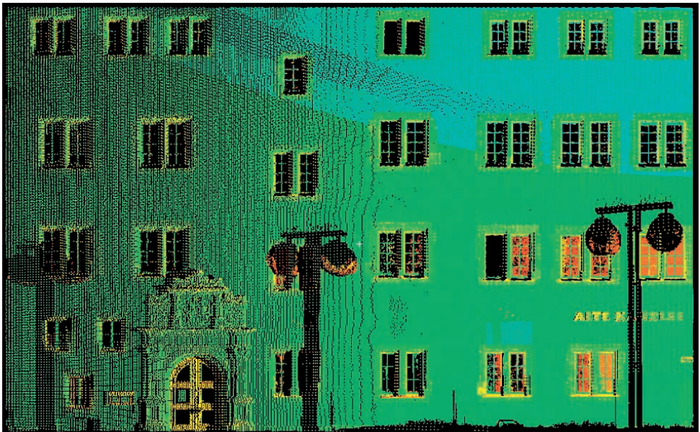
Fig. 2: 3D point cloud as used for the geometric refinement of the corresponding building facade.
