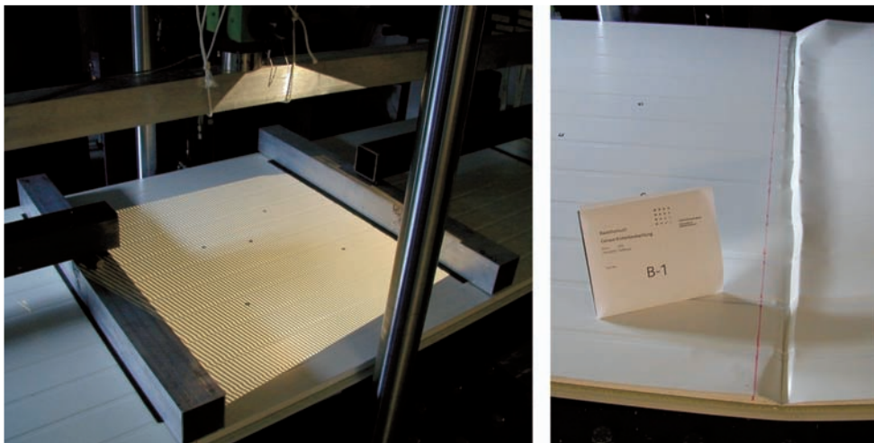
Fig. 2: Setup for six point bending test (left); sandwich after wrinkling failure (right).
