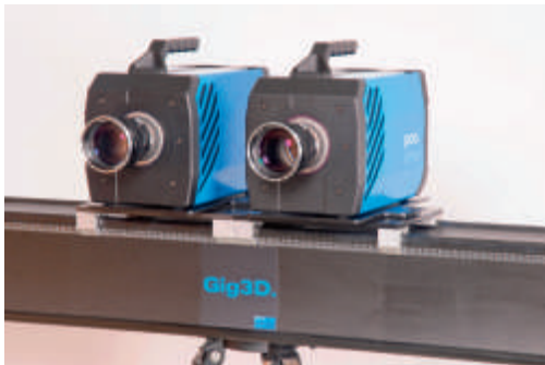
Fig. 2: a) pco.dimax in a stereo rig setup, b) With mounted beamsplitter.
