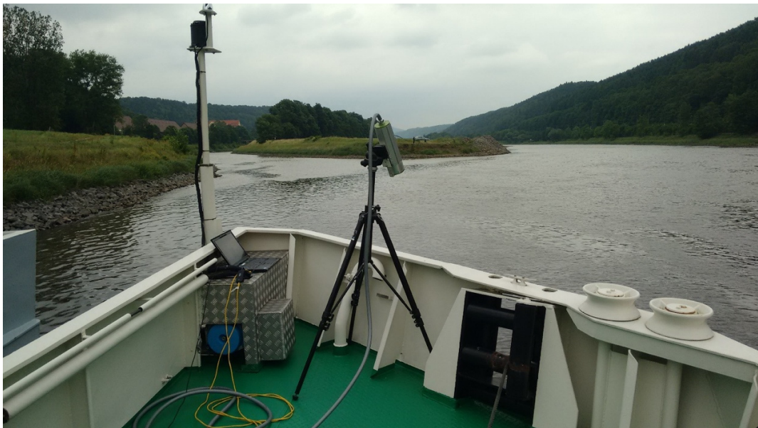
Fig. 1: Hyperspectral sensor mounted on the bow of the research ship
