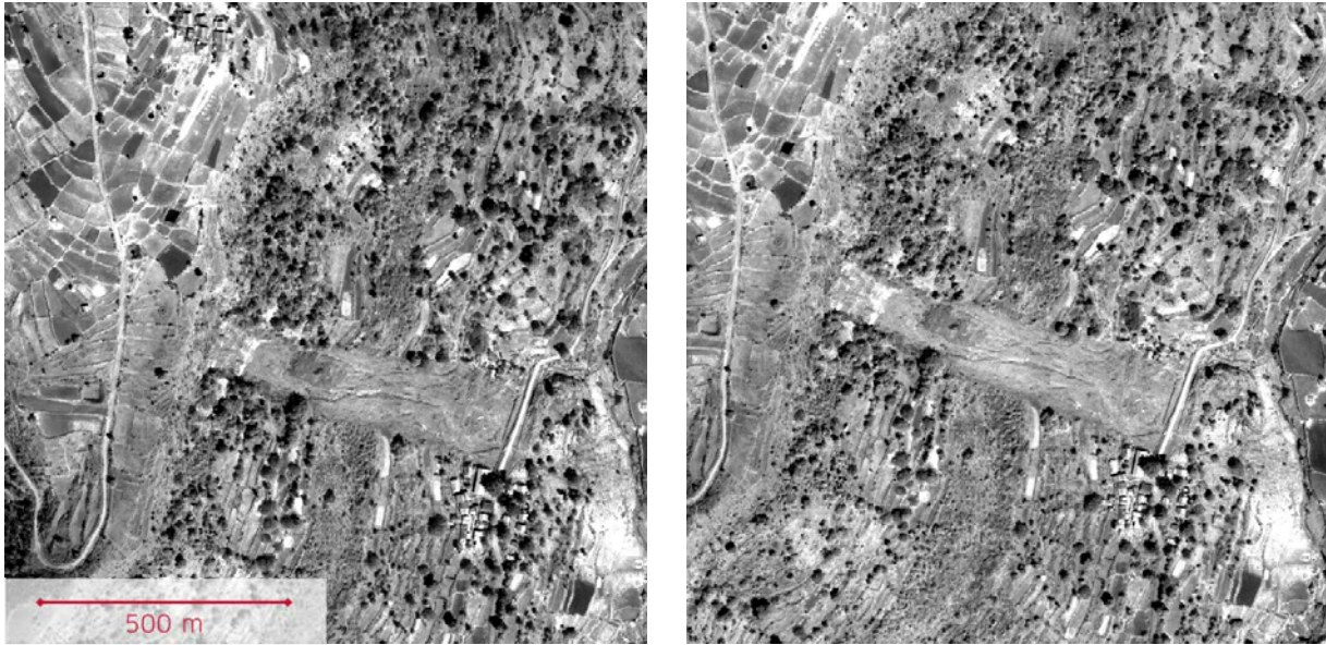
Fig. 1: Pléiades panchromatic stereo pair of the Malin landslide area, used to run the photogrammetric generation of a point cloud from optical imagery (subset, GSD 0.5 m). Left: Pléiades 1A, acquired 8 Feb 2015, incidence angle 21.6°. Right: Pléiades 1B, acquired 9 Feb 2015, incidence angle 1.9°.
