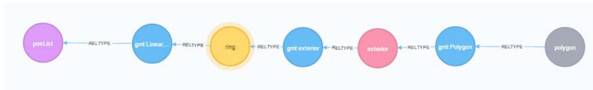
Fig. 3: GML polygon represented as a chain of nodes in Neo4j database which corresponds to its original XML tree structure.
