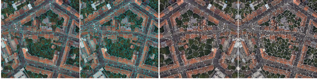
Fig. 1: Superpixel segmentations with different capacity. First two images are segmented by SEEDS and the last two by SLIC.
