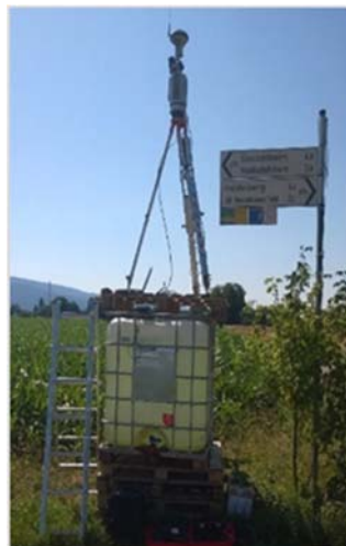
Fig. 1: Scanner set up on stable barrel for elevated scanning at a height of 3.6 m, located at one edge of the monitored maize field.
