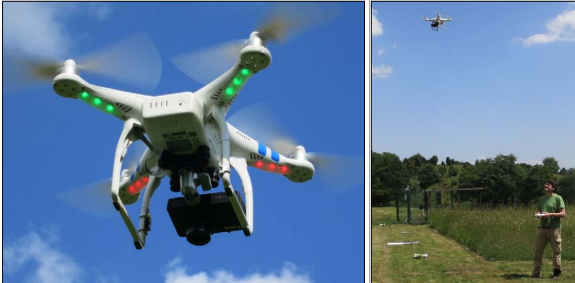
Fig.1: left DJI Phantom 2 with the mounted Canon Powershot 110; right the UAV imaging system in air at the RGE
