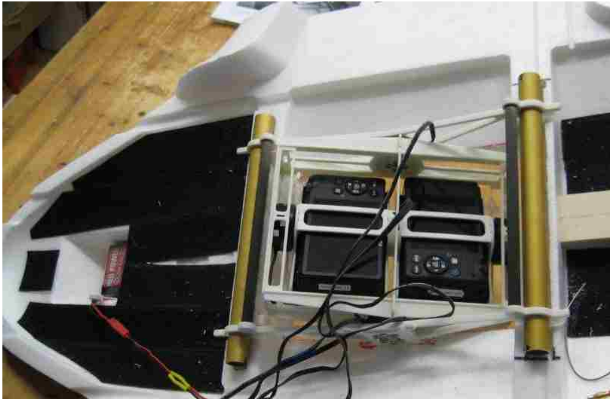
Image 1 2-axis dual-camera gimbal in a roll and pitch inclined fixed wing airplane body
