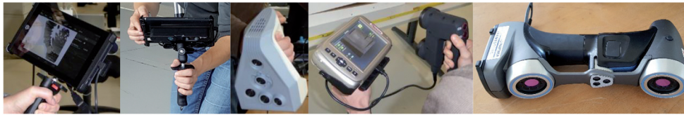
Fig. 2: Examined handheld scanner systems (from left): DPI-7, DPI-8, Artec Spider, Mantis Vision F5 SR, and Creafom HandySCAN 700.
