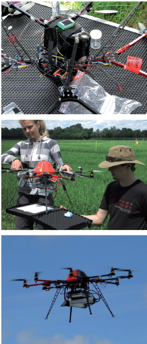
Fig. 1: Top: MK Oktokopter is prepared for a flight campaign with the Rikola hyperspectral camera, middle: Cubert UHD185 Firefly is calibrated against a white panel before take-off, bottom: UHD185 in the air mounted on a MK Oktokopter.
