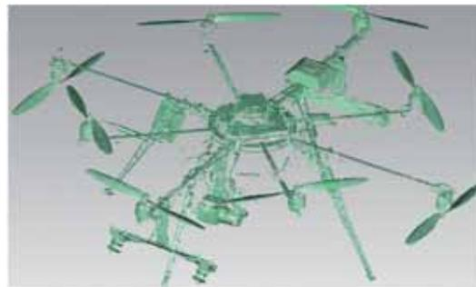
**Fig. 6:** Point-cloud of a laser scan, which has been used for the system calibration.
