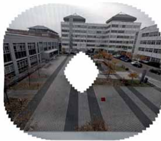
Fig. 9: Image mosaic generated by applying the angles \phi , \theta and \psi and additional boresight corrections for the oblique images.
