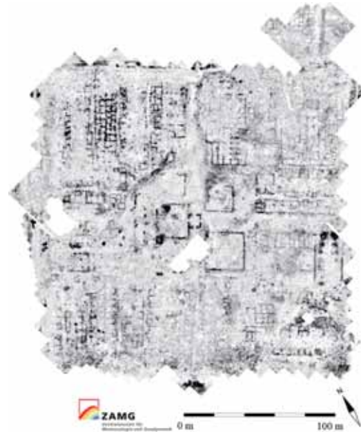
Fig. 4: Qreiyeh. Exemplary depth slice of 20 cm – 30 cm depth. Sensors & Software PulseEKKO 1000 with 900 MHz antenna, GSSI SIR-3000 with 400 MHz antenna, and Sensors & Software Noggin with 500 MHz antenna; sample interval: 5 cm x 25 cm or 50 cm (after: SEREN et al. 2009).
