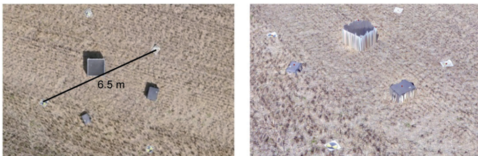
Fig. 8: Experimental design of accuracy assessment (left: photo, right: DEM): Reference points are four GCPs, two different sized Peli Cases and 4 corners of the UAV transport box.
