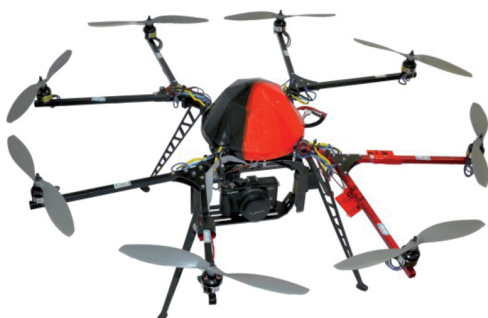
Fig. 3: MK-Oktokopter by HiSystems GmbH mounted with RGB sensor.
