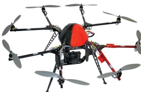
Fig. 3: MK-Oktokopter by HiSystems GmbH mounted with RGB sensor.
