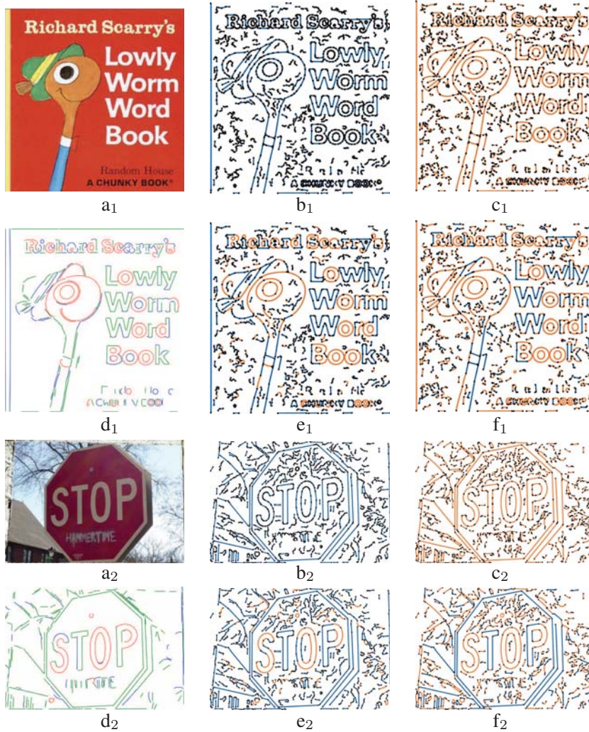
Fig. 3: Pre-segmentation circlePeucker vs. Douglas-Peucker (Best viewed in colour). a_* : Given images as used in PATRAUCEAN et al. (2012). b_* : Pre-Segmentation using Douglas-Peucker. c_* : Pre-Segmentation using circlePeucker . e_* and f_* : Final segmentation using b_* and c_* , respectively. d_* results by ELSD. Colours, see Figs. 1 and 2.
