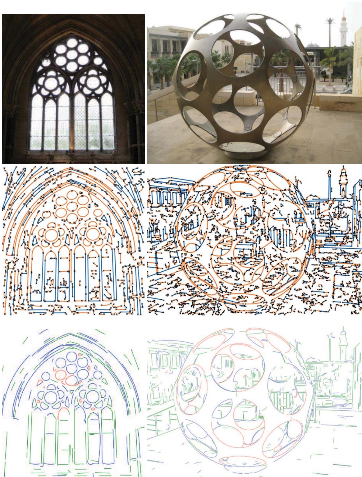
Fig. 5: More results on real images (Best viewed in colour). Left: Gothic window. Right: cropped icosahedron. From top to bottom: given image, our final result using circlePeucker for pre-segmentation, result of ELSD. Colours, see Figs. 1 and 2.
