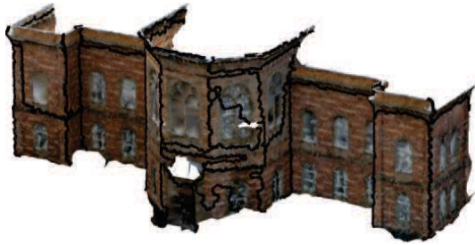
Fig. 8: Surface segmentation on a visually reconstructed, meshed point cloud.
